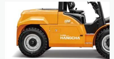
Designed for high load capacity, minimizing the risk of rear tipping and ensuring more stable operation.
