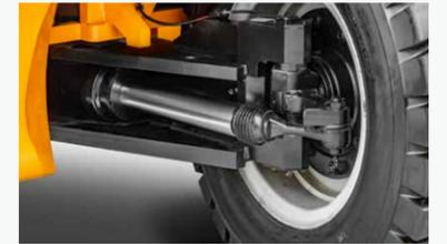
Utilizes internal combustion truck structures, including the frame and front/rear axles, paired with large tires for increased ground clearance, making it more suitable for outdoor operations.
